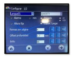
TO INCREASE THE ENGRAVING DEPTH, KEEP THE + BUTTON, PLACED ON THE RIGHT OF "DEPTH OFFSET" LINE, PRESSED UNTIL THE MAXIMUM VALUE WILL BE REACHED.
